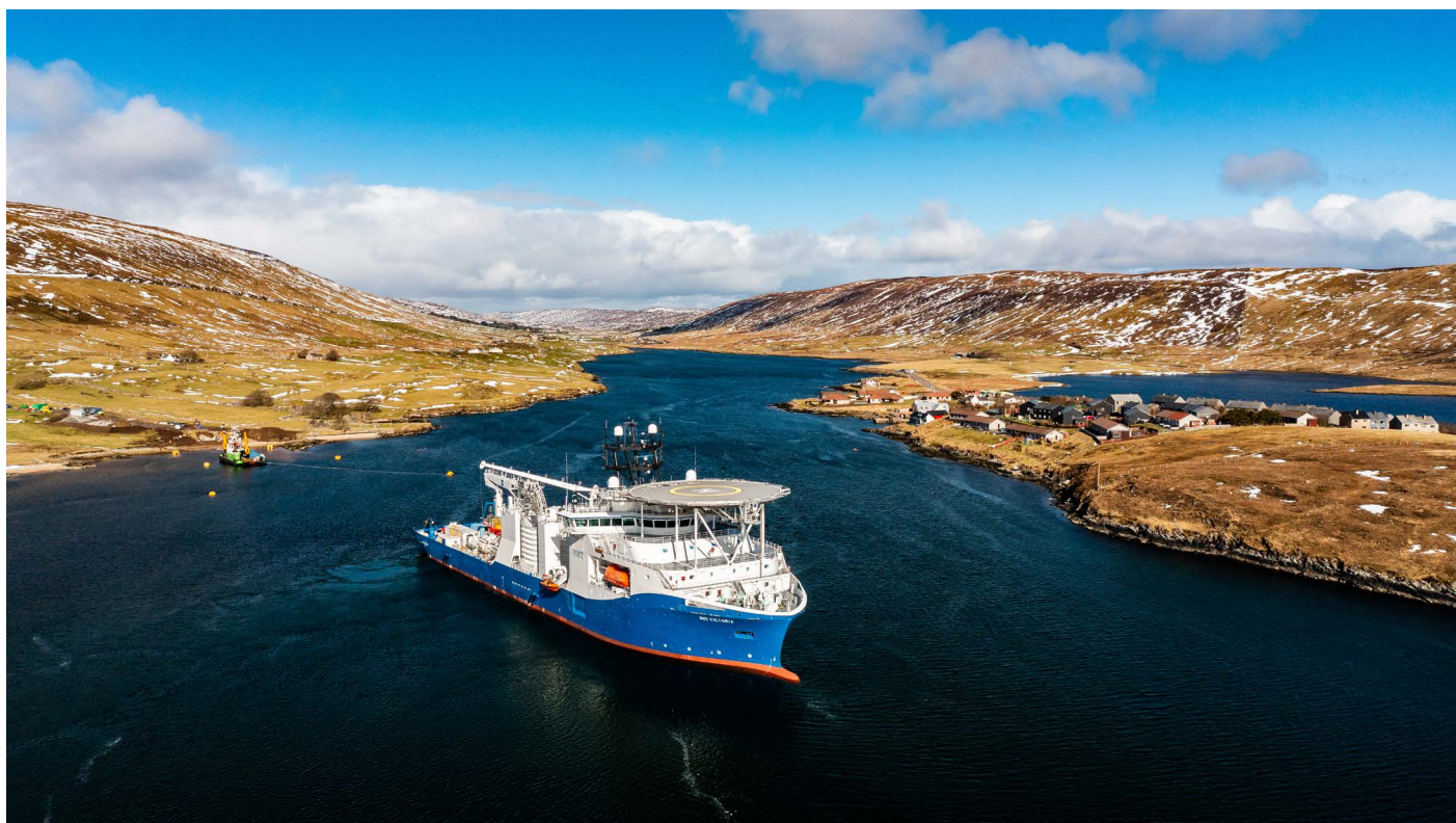
An SSE Transmission vessel prepares to pull an HDVC cable to carry electricity from Shetland to mainland Scotland.
